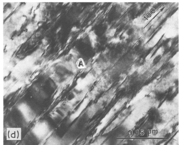
Figure 3 TEM micrograph of deformed material. (a) 25°C sample. Note distortion of the twin lamellae due to dislocations (A). (b) A different grain in the same sample showing an irregular fracture (A) and stacking faults (B). (c) 500°C sample. Dislocation arrays (A) are on (001) planes and deformation twins (B) are on {110} planes. Insert shows the sample with a 10° tilt toward the [001] to reveal the dislocations going through the foil. (d) 800°C sample. Note that faint residual contrast of the {110} twins (A). (e) Different grain in the 800°C sample showing a polygonal structure (see the text).
